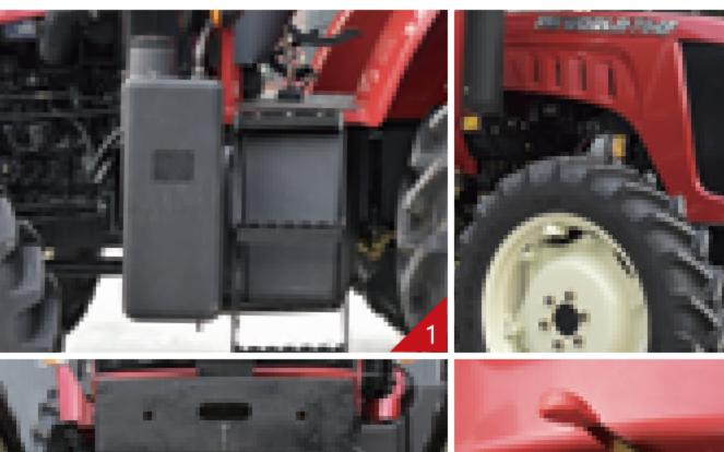
115L large integral fuel tank provides long time working.
